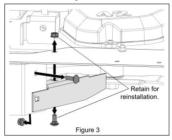
6. Reinstall 5/16" x 3/4" round head square neck bolt and flange nut to prevent debris from escaping from cutting chamber. See Figure 4.
