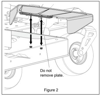
Remove one 5/16" x 1" and one 5/16" x 3/4" round head square neck bolts and two flange nuts retaining deflector strip and remove deflector strip. Retain deflector strip and 1" bolt and one nut for operation without mulch kit and 3/4" bolt and nut for reinstallation. See Figure 3.
