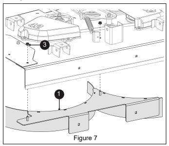
Secure baffle to front of deck with two 5/16" x 3/4" round head square neck bolts (item 2) and two 5/16" locking flange nuts (item 3). See Figure 8.
