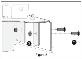
Secure baffle to rear of deck with one 5/16" x 3/4" round head square neck bolt (item 2) and one 5/16" locking flange nut (item 3). See Figure 9.
