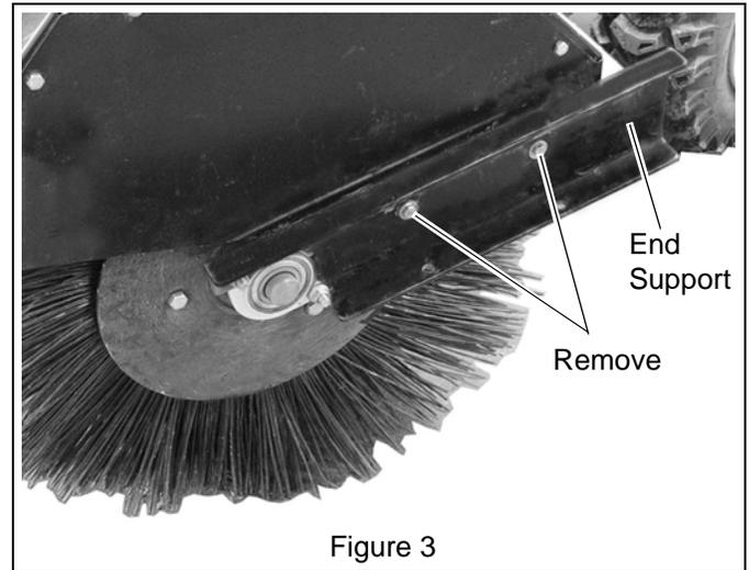
3. Tip unit backward onto handlebars. Bolts from end support will fall out and brush will stay on ground. See Figure 4.
