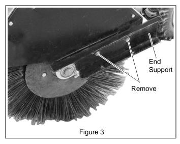
Tip unit backward onto handlebars. Bolts from end support will fall out and brush will stay on ground. See Figure 4.
