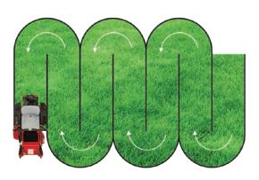
A zero-turn mower will allow you to cut your lawn efficiently as you can turn 180° at the end of a mowing row. There is no need to drive over previously cut areas or waste time backing up to manoeuvre into position for the next pass
