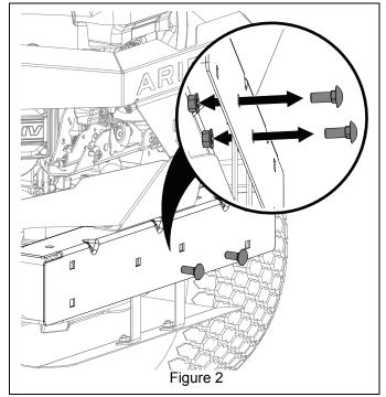
Position hitch plate (item 1) on bumper and retain rear face with two round head square neck bolts just removed and two 3/8" locking top flange nuts (item 3). Install bolts with threads facing out. See Figure 3.
