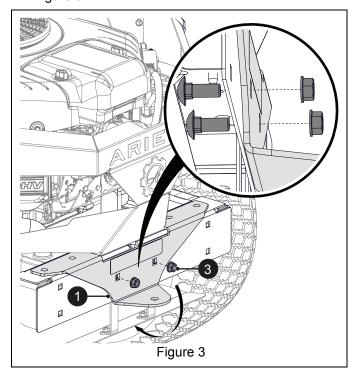
Retain top of plate face with two 3/8" x 3/4" hex bolts (item 2) and two 3/8" locking top flange nuts (item 3).
