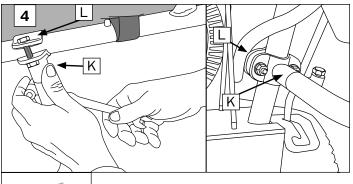
Continue adjusting and tightening the mounting post brackets [K] and [L] on the machine and on the cab. Keep adjusting until bottom of the cab is level with the ground and that it looks centered.
