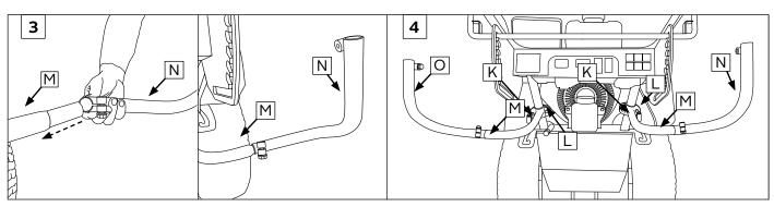
Next, slide the right outer mounting post [N] into inner mounting post [M]. Repeat on the left side by mounting part [O] on top of part [M]
