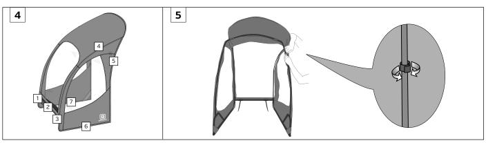
Attach rip-and-grip tabs in the proper sequence. Fabric will be tight to the frame and hoop assemblies.
