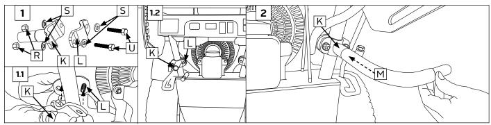
Assemble the upper clamp mounting post [K] to the top plate [L] on the post on your machine (See figure) Secure with two washers [S], two 35 mm hex bolts [U] and two hex nuts [R].
