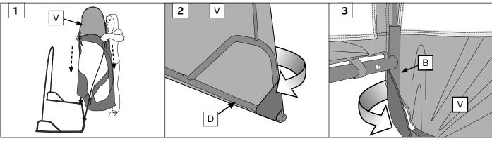
Slide the pocket in the top of the skin [V] over the installed front hoop assembly.
