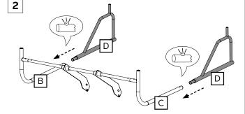
Slide the two support brackets [X] onto the center mounting bar [A] These will be adjusted to attach to your machine later.
