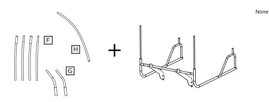
The back hoop side poles  $[\mathsf{F}]$  are designed to fit together by matching tapered ends as shown.
