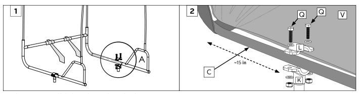
Before mounting assembled cab onto the snow thrower, loosely secure a mounting post [K] and the upper clamp top plate [L] together.
