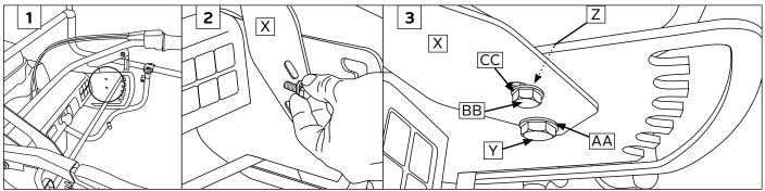
Locate the holes in the machine. Tip: Dropping the handlebars on the machine may make it easier to align the holes. Align the holes in the support bracket [X] with the holes on the machine.
