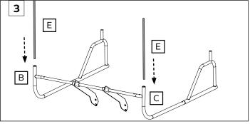
Insert the front poles [E] onto the upright ends of the side mounting bars [B, C].
