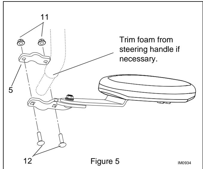
6. Tighten fasteners to keep assemblies in position but still allow adjustment.
