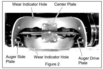
6. Secure auger paddles to center plate as shown in Figure 3. Torque hardware to 5.7 N•m − 10.2 N•m (50 lb-in − 90 lb-in).
