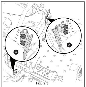
6. If not pre-installed, secure brackets to headlights (item 2) with included hardware. DO NOT completely tighten hardware until headlights are adjusted. See Figure 4.
