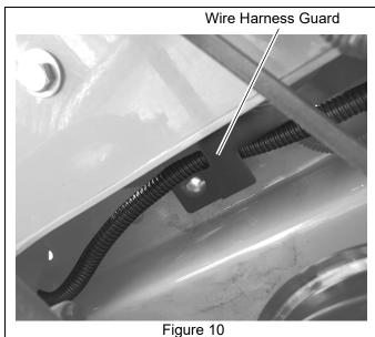
14. Continue to route headlight wire harness end out through left side of frame and above left damper / fender mount bracket. See Figure 11.
