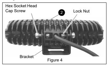
7. Secure each headlight to mounting brackets with included hardware. Headlights can be mounted either horizontally or vertically depending on preference. Do not fully tighten. See Figure 5.
