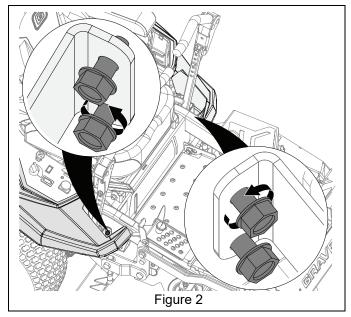
5. Position left headlight mounting bracket (item 3) and right headlight mounting bracket (item 4) behind pivot bracket screws and tighten screws. See Figure 3.
