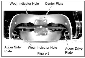
Secure auger paddles to center plate as shown in Figure 3. Torque hardware to 5.7 N•m – 10.2 N•m (50 lb-in – 90 lb-in).
