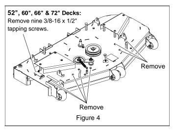
6. Remove bolt and washer retaining blades to spindle and remove blades. Retain all hardware. Save blades for operating unit without mulch kit. See Figure 5.
