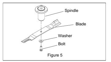
Install mulching blades with spindle hardware removed in Step 6. Torque blade bolt to 115 – 120 lbf-ft (156 – 163 N•m).  Install left mulch baffle (Item 3), right mulch baffle (Item 4) and discharge mulch baffle (Item 2) on the mower deck with eight 5/16"-18 nyloc flange nuts (Item 5). See Figure 7.
