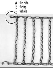
Lay chain straight with the open sides of the cross chain hooks facing up. The open sides of the cross chain hooks must be facing away from the tire when the chain is installed. Make sure all twists are out of the chain assembly.
